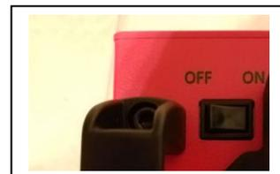
3.6) Push the meter down and hold until the test is complete and the display reads “Done Lift Meter” Should read DCOF = 0.000
