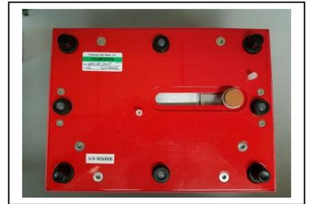
**Do not press hard or attempt to move the assembly by sliding the mechanism or side to side. This will damage the load cell.**
